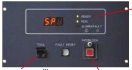
RJ-45 Ethernet<sup>™</sup> port is used for local toolbox connection
