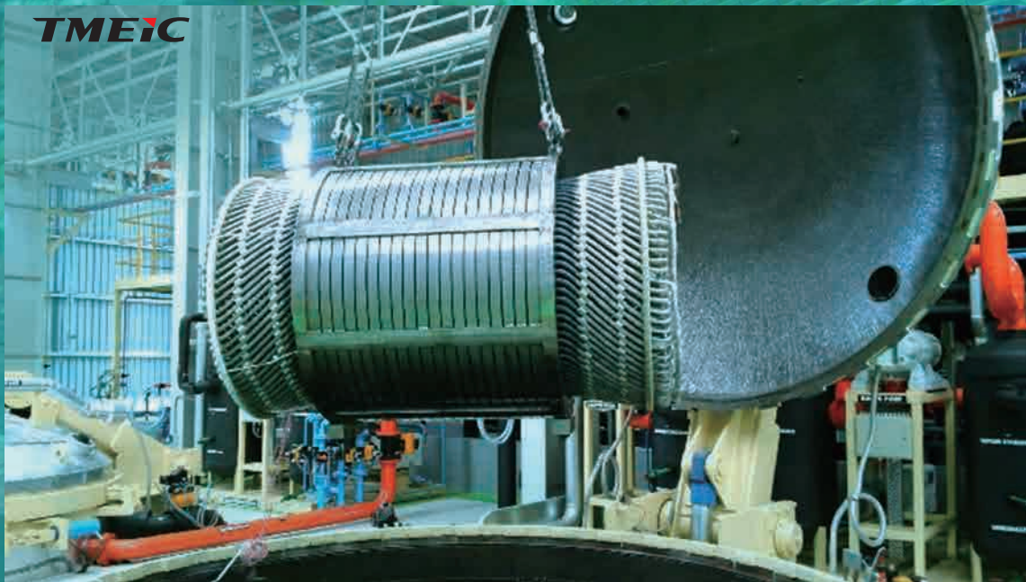
Installing stator in VPI tank
