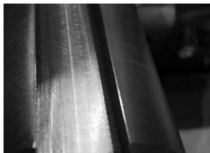
After finishing keyway
