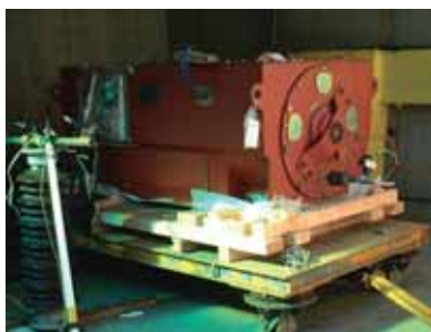
Hydrogen gas test
